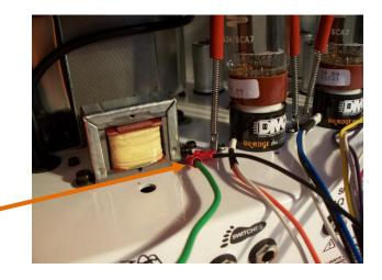
Green earth wire connected to amplifiers chassis
