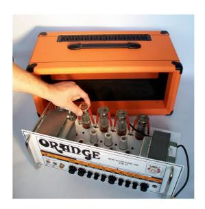
Very carefully remove each output valve from the valve socket. Slacken or remove any valve retainers where necessary. Hold the valve at the valve base and gently move or rock the valve in a circular motion whilst applying an upward force.
