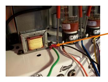
Zero volt wire Connected to amplifier's chassis
