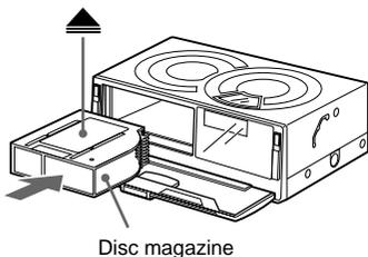
Insert the magazine (which has been taken out of the unit) firmly with the **▲** mark visible on the top side.
