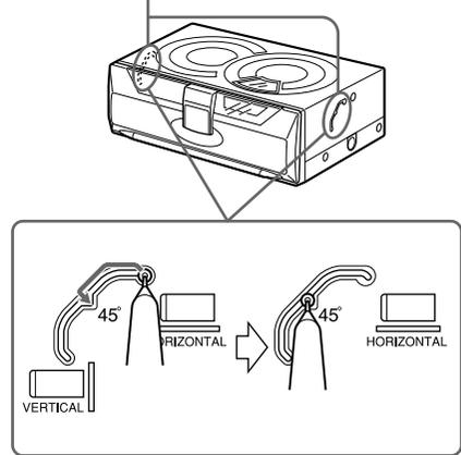
Insert a pointed object such as a screw driver or ball-point pen, etc. into the low spot of the lever and slide the lever to the position from among HORIZONTAL, 45°, and VERTICAL positions.
