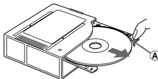
To remove a disc, pull part **A** in the direction of the arrow as illustrated.
