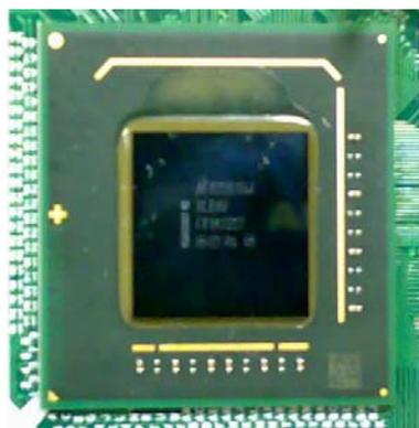
The Intel® System Controller Hub US15W is a low-power chipset in one small 22x22 mm package, It combines the Intel® Graphics Media Accelerator 500, memorycontroller, and I/O controller in a single-chip solution while featuring advanced 3D graphics and extensive I/O capabilities such as USB2.0,SDIO and PCI Express. It supports Intel® High Definition Audio and hardware video decode acceleration, a 400/533 MHz CMOS front-side bus, dual independent display.
