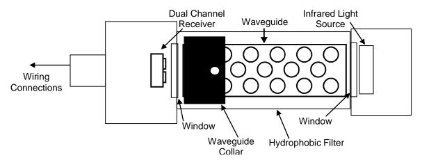
Using a dual channel receiver there is no need to use any special lenses or beam splitters to achieve the different measurement bands.
