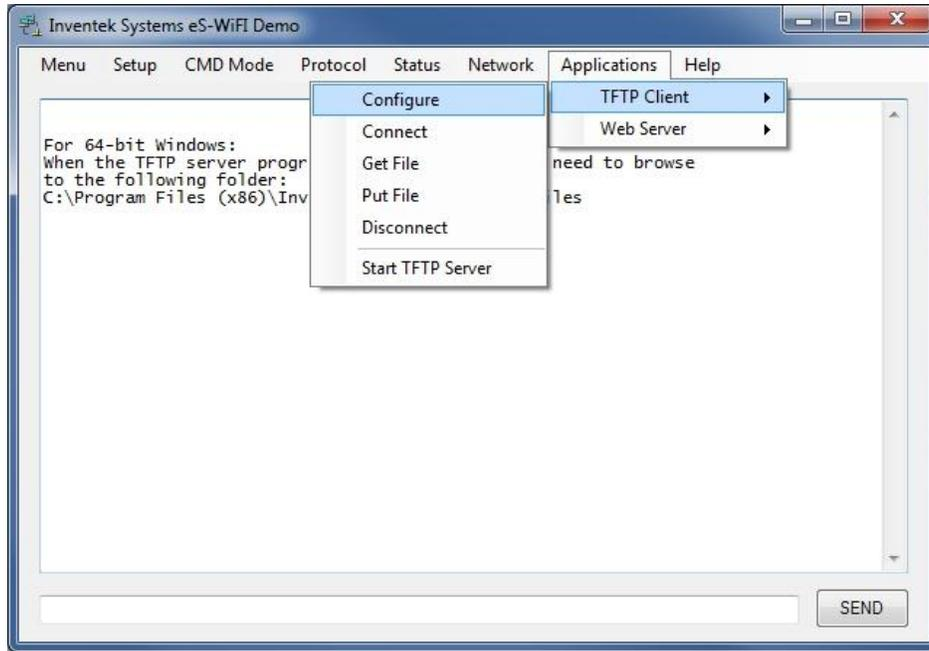
Now enter the IP Address of TFTP Server (from above it would be 192.168.1.154). You only need to change the defaults when using different files. Once entered click the OK button.
