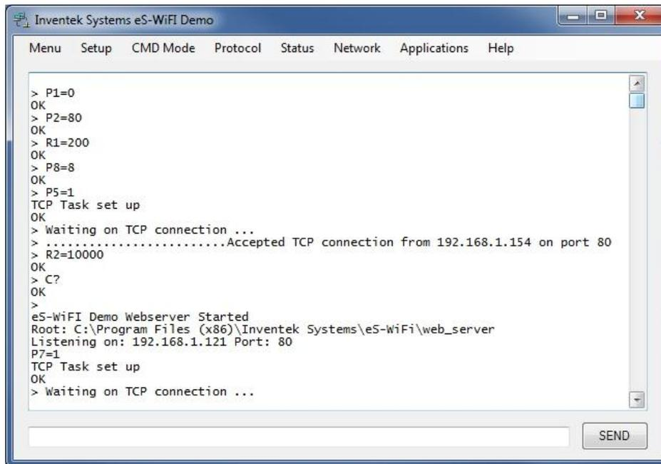
By entering the eS-WiFi EVB IP address in the browser and pressing the enter key the browser requested a connection. We see the Accepted response for the browser at IP address 192.168.1.154 on port 80.
