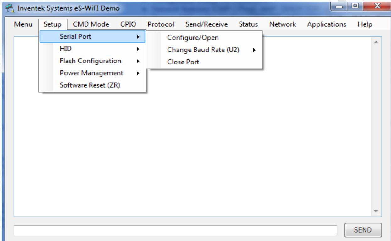
You will now configure the VSP (Virtual Serial Port) connection the EVB. You will need to determine what COM port is attached to the EVB. This can be done by using Windows Device Manager. In this case, COM54 is the port connected to the EVB.
