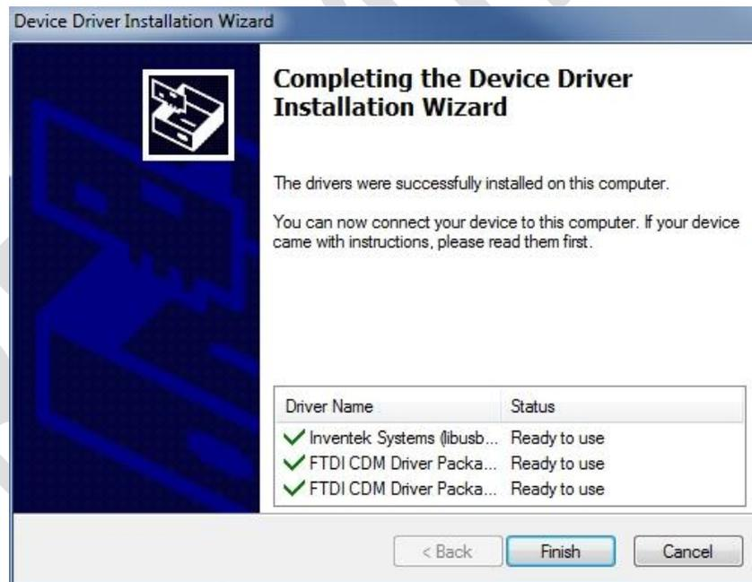
Connect the ISM4319-M3-EVB board to a USB port on your computer. Once the Install device driver software message have completed the EVB is ready for use.
