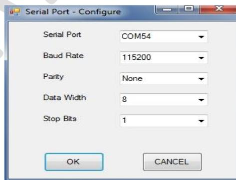
Click the OK button and press the Reset button on the EVB (SW2). You will now see the reset banner. You can also perform a soft reset with the drop down menu under SETUP.
