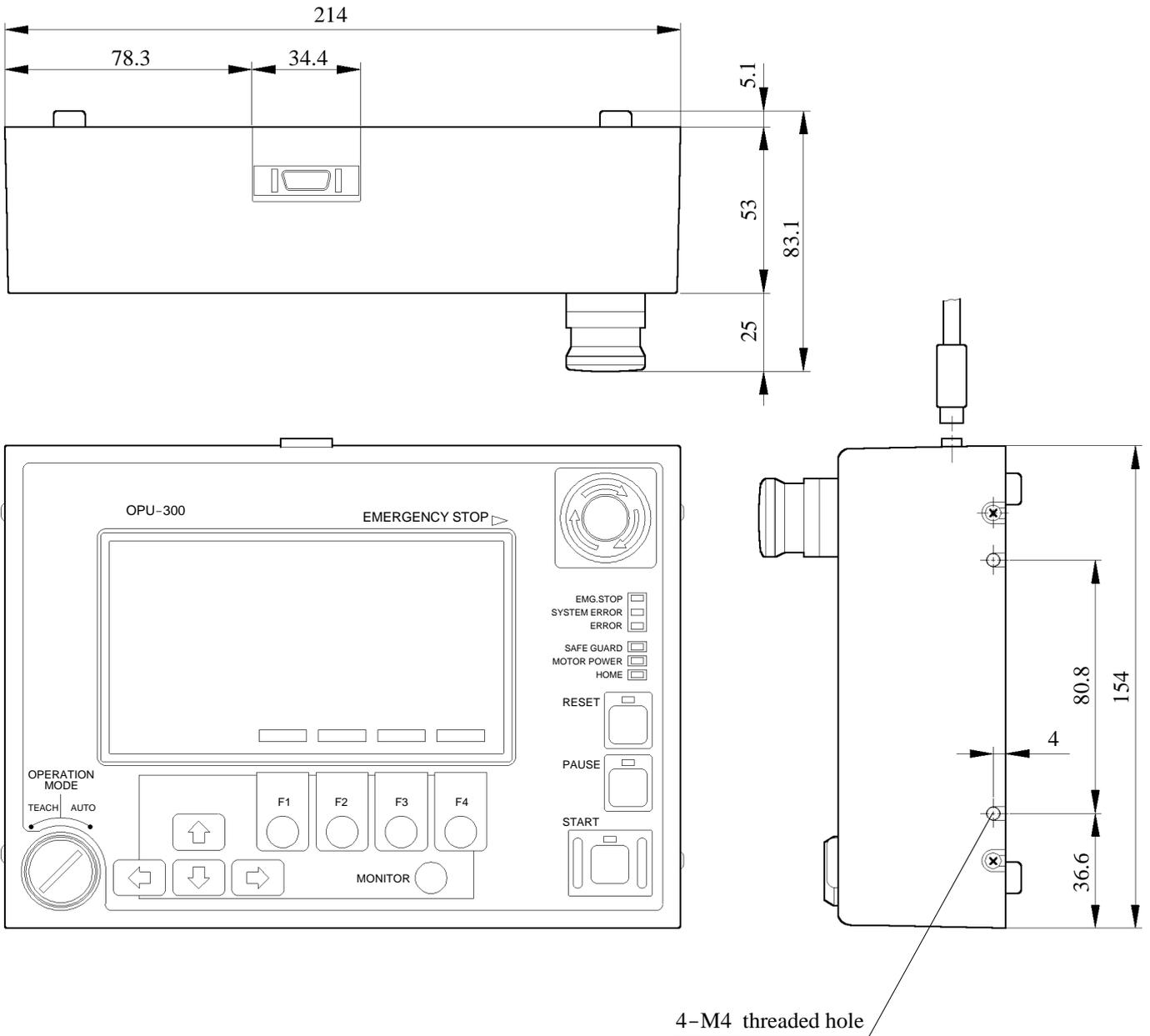
Figure 5.1 External dimensions (mm)
