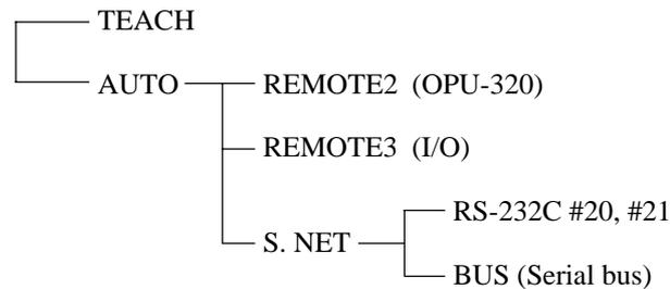
You can switch between the AUTO mode and TEACH mode by turning the key of the mode selector switch on the OPU-320.
