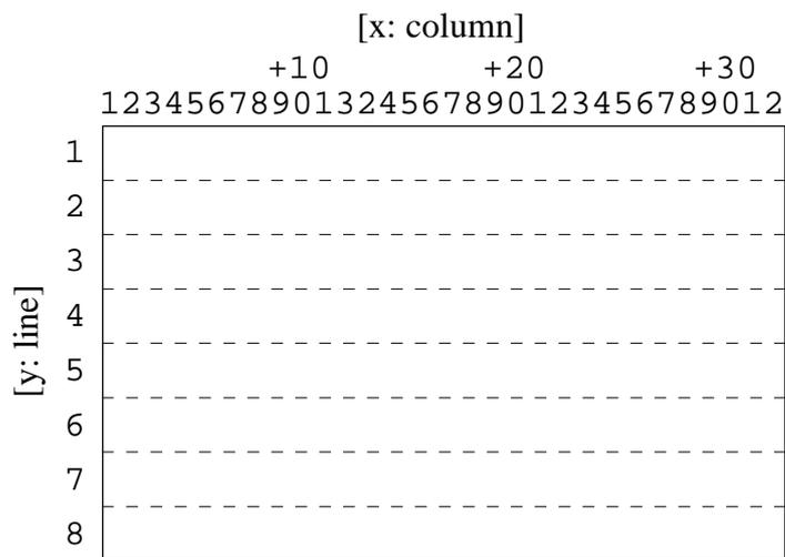
Figure 4.1 OPU-320 screen configuration
