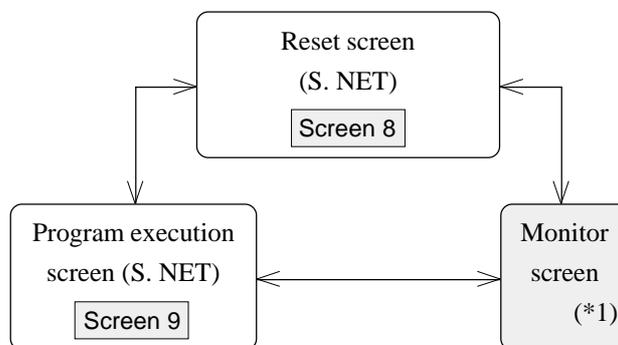
Figure 2.3 AUTO mode (S. NET) state transition diagram
