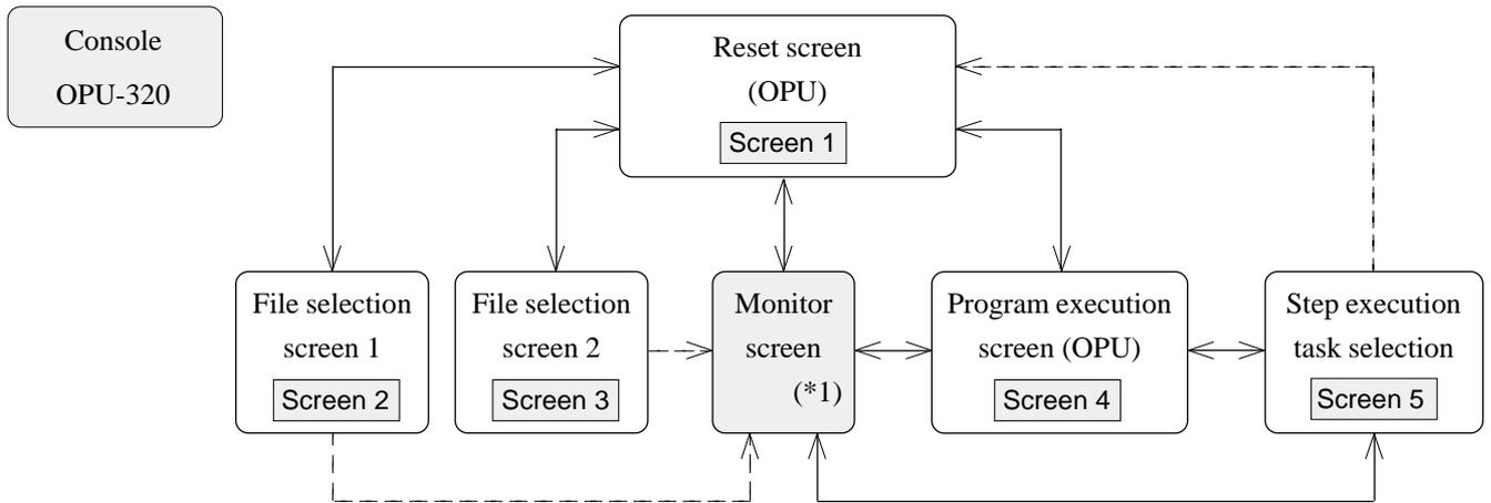
Figure 2.1 AUTO mode (OPU) state transition diagram
