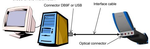
For the USB optical cable (option), install, if necessary, the recognition software on your PC (see CD-Rom MANUAL provided).
