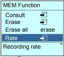
• Validation of Rate with the key opens a menu for setting the required recording rate in hours, minutes and seconds:
