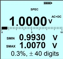
In AC+DC, the specifications are calculated only if the frequency can be measured (see §. Secondary Functions) and is > 45 Hz.
