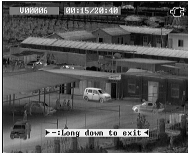
In the above picture, the file name, recording time and left recording time are displayed. Long press “-” to stop the video taking.
