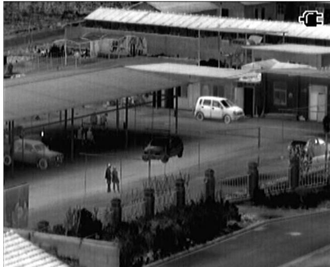
When the thermal imager works with the enclosed Li-ion battery, a battery mark will present in the right corner of the screen as the below image shown.
