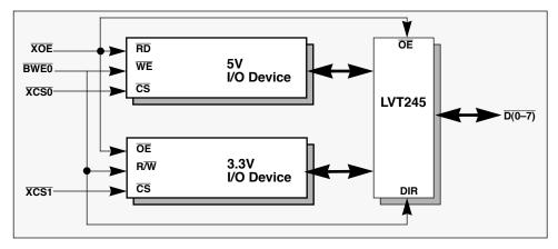
Figure 7. Buffered I/O Connections
