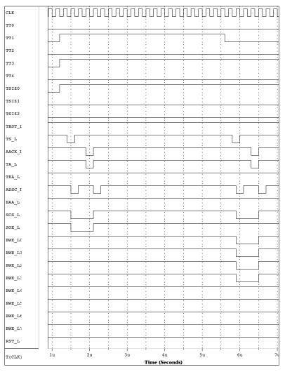
Figure 14. Pipelined Burst SRAM-Single-Beat Read/Write
