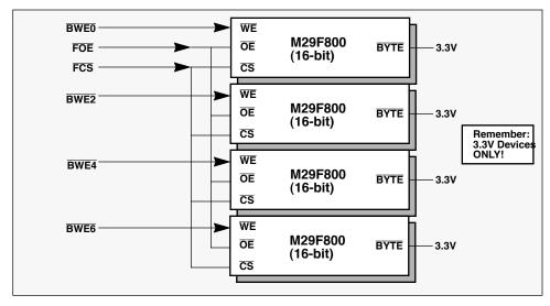
Figure 5. Flash Memory Connections
