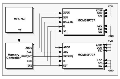
Figure 4. Pipelined Burst SRAM Memory Connections
