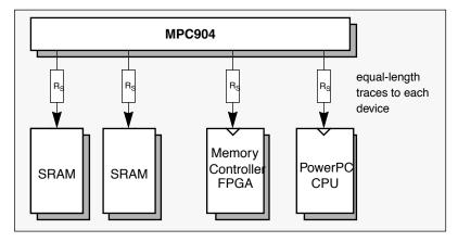
Figure 19. MPC904 Clock Connection
