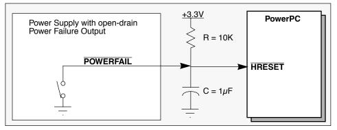
Figure 21. Simple Reset Controller
