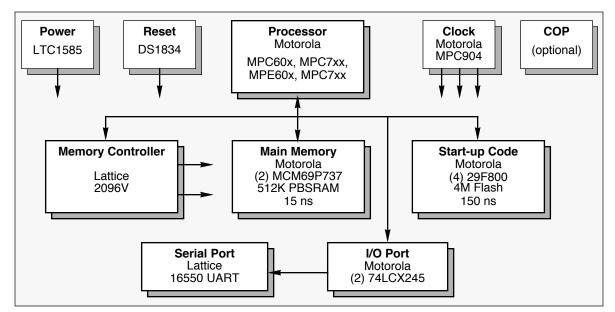
Figure 1. Typical Minimal System Block Diagram
