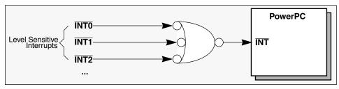
Figure 26. Simple Interrupt Merging
