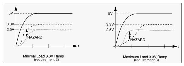
Figure 24. Power Supply Sequencing
