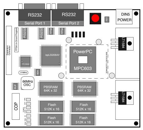
Figure 31. Excimer Minimal System Board
