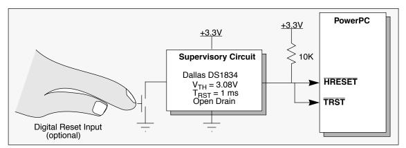
Figure 20. Reset Using Supervisory Controller
