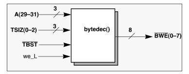
Figure 10. Byte Write Enable Module
