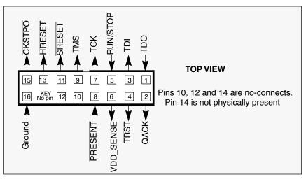
Figure 28. COP Connector Diagram
