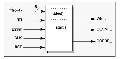
Figure 9. Start Detector Module
