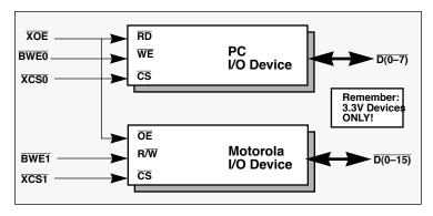
Figure 6. I/O Connections
