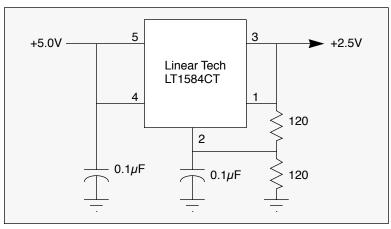
Figure 22. Excimer Linear Power Supply
