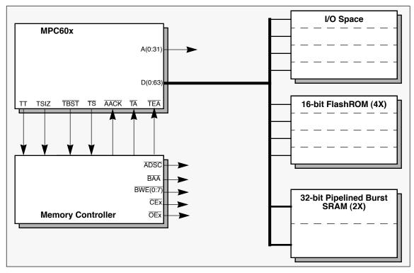
Figure 3. Minimal System Memory Architecture
