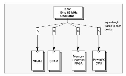
Figure 18. Simplest Clock Connection
