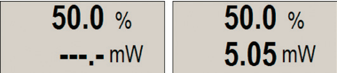
Figure 9. Power meter panel: Left - "Use absolute power measurement units" checkbox is set in "Options->Preferences", right - checkbox is unset.
