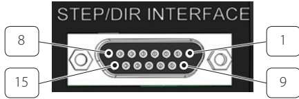
Figure 19. "STEP/DIR INTERFACE" 15 pin D-SUB female connector on the controller case
