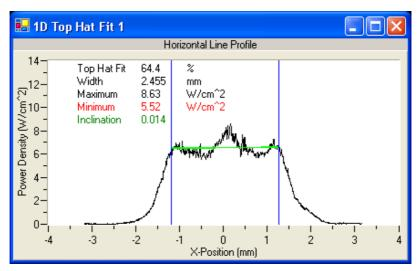
Figure 15: Top Hat fit example with Pass/Fail option active
