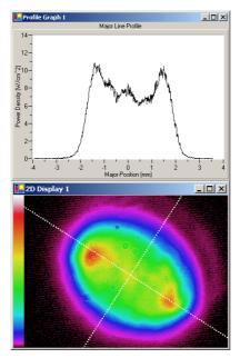
Figure 13: Example of a Line Profile along the Major Axis
