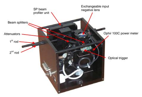
Figure 1: View of components of Beam Cube Assembly
