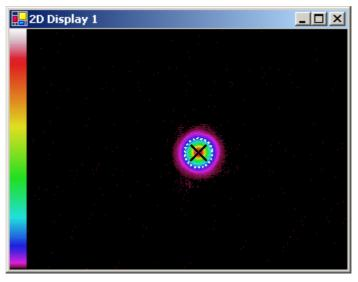
Figure 11: Example of 2D Display with Centroid and  $4\sigma$  beam width Markers selected
