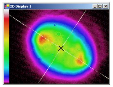
Figure 20: Major and Minor lines drawn through the centroid of a rotated laser beam
