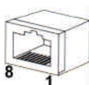
RJ45 Pin Locations (For RS232 or Ethernet)
