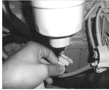
Figure 34 - Removing the water in fuel presence sensor
