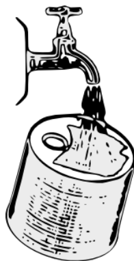
Figure 32 - Sea water filter cleaning under running water
