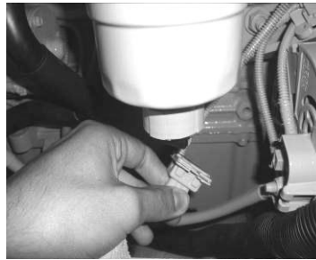
Figure 30 - Removing the water in fuel presence sensor
