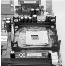
2. Position the heatsink and fan onto the retention mechanism.
