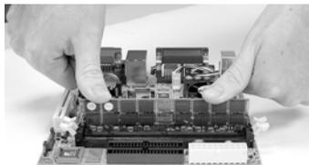
3. With both hands, press the SDRAM module down into the DIMM slot so that the white retaining latches rotate up and secure the module in place (see picture below).
