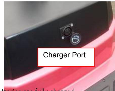
Recharge the battery only when the scooter is switched off. When the battery indicator shows low power, recharge the battery.
