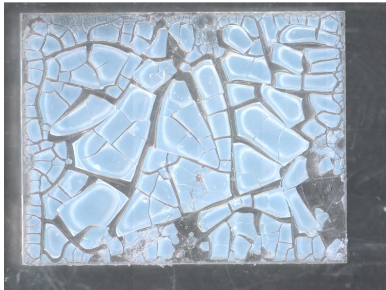
FIGURE 4.11: 100ml Amorphous GadOx solution on a quartz substrate. Sufficient cracking can be seen due to moisture retention between the quartz and the GadOx
