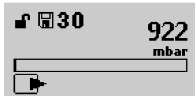
Fig. 20: Evacuation status display (047)
