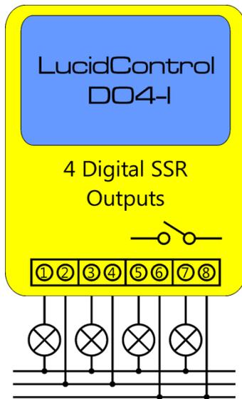
Fig. 2 DO4 Module with Solid State Relays
