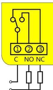
**Fig. 8 Relay Output**
