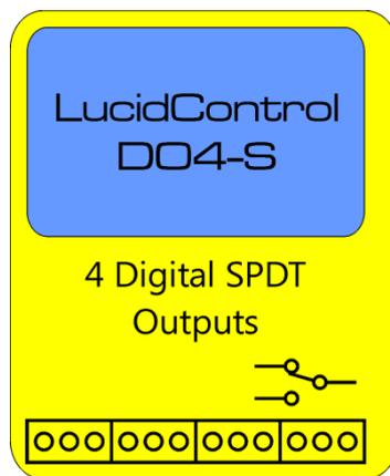
The DO4-S module uses 4 mechanical “single pole double throw” (SPDT) relays. This relays have the advantage of behaving like mechanical switches closing a circuit. This allows not only switching of electrical power but also switching of measurement signals e.g. from a temperature sensor which would be distorted by using solid state relays.
