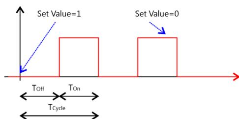
**Fig. 9 Duty-Cycle Mode**
