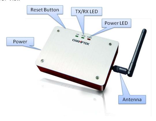
Power LED – On when reader is powered.
