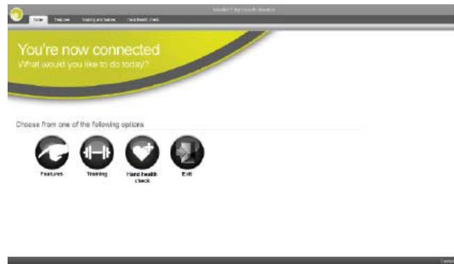
**Features** allows the set-up of the i-limb digits and is where triggers are linked with with grip patterns and gestures.
