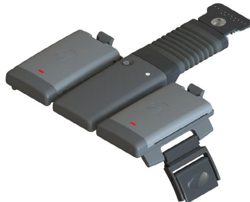
The Wristband is switched on and off via the grey button on the central panel. The light sequence is as follows:
