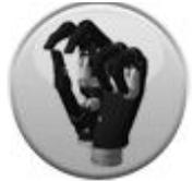
Thumb 3 Jaw Chuck (Tripod) Opened
