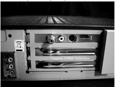
For the best sound effects, when you are going to enjoy music and movies only by two speakers system, we recommend you connecting a two channels DAC device to the Evolution-I through the coaxial S/PDIF interface. Of course, you can directly connect the FRONT analog output to your stereo amplifier from Evolution-I if you have not a DAC device.
