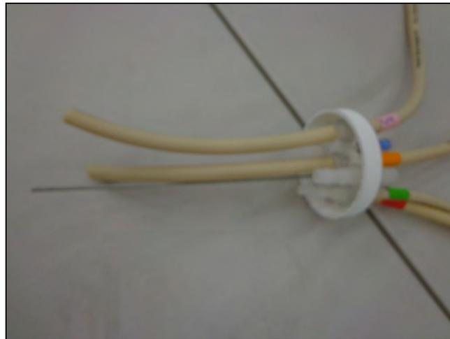
**15.** Seal the 1/2 inch Barb Fittings that are not in use with caps. {30603} This is to maintain the system's sterility.
