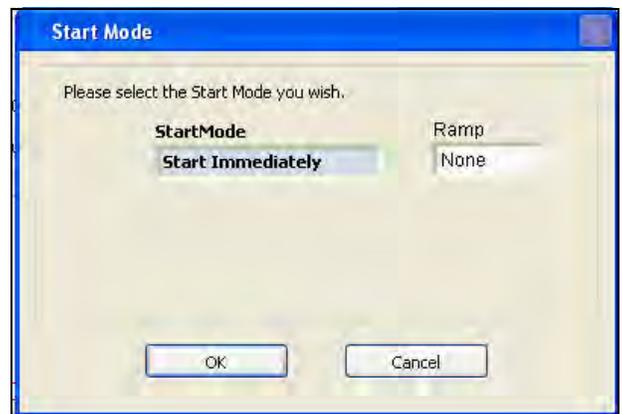
Ramp allows the user to select the speed at which the pump will deliver. There are options in increments ranging from very slow to very fast. “None” is also an option for type of ramping.
