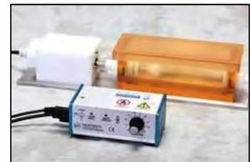
The rotating double chamber is specifically designed for cell seeding and culturing both surfaces of a tubular matrix. The **intraluminal** and **extraluminal** flow paths may be connected or maintained separately. The hollow organ chambers allow seeding and culturing of different cell types on either side of the tubular structure, providing homogeneity. The design allows for enhanced oxygenation and mass transport between the medium and cells.
