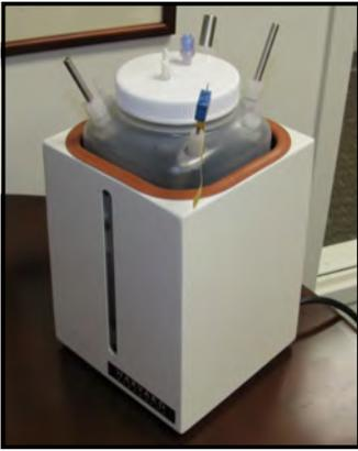
The heater is used to maintain temperature throughout the system to **emulate physiological conditions**.
