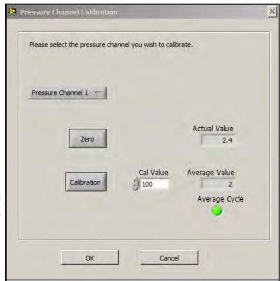
**WARNING:** You must have a pressure measurement device and a way to increase the pressure. IF you press the calibration button and do not have a way to measure the actual pressure you will establish a false reading and not be able to use it (typically 100 mmHg).
