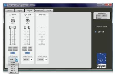
The combo boxes at the bottom of the page allow connecting each physical output of the VX442 (two pairs of analog outputs and one pair of digital outputs) to one of the six stereo sources available on the card:
