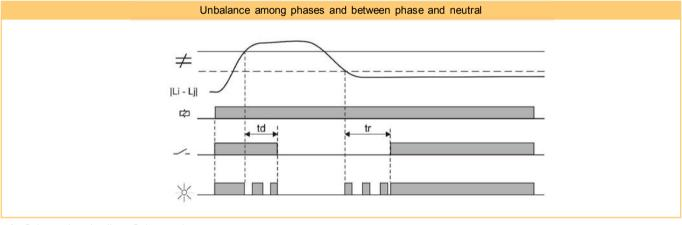
td = Delay on detection // tr = Delay on release
