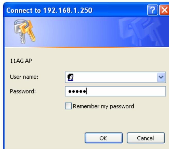
In order to configure the Wireless 11ag AP, you must input the password into the **Password** box and leave blank on the **User Name** box. The default password is **"admin"**.
