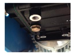
To refill the crankcase oil, remove the orange breather plug on the top of the high-pressure pump. Insert a long stemmed funnel through the circular inspection port and add 350ml (12 ounces) of oil.
