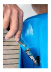
3. Remove the clear plastic spiral intake hose from the hose pocket on the Pressure Supply Unit and remove the cap.
