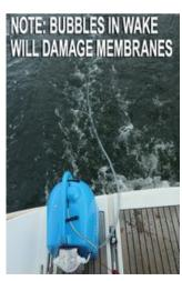
We recommend sliding the intake cap up the intake hose and securing it on board the vessel so that the end of the intake hose can sink sufficiently below the surface.
