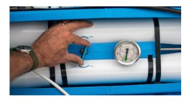
Never exceed 58 bar (850 psi). If you over tighten the pressure control valve, a relief valve in the Pressure Supply Unit will release and water will recirculate within the unit. This prevents damage to the RO membranes from excess pressure. However, prolonged operation of the relief valve can damage the unit.
