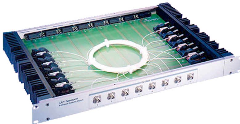
Figure 6 – Mounted Butterfly Packages and Fiber Optics
