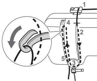
**7** Make sure you guide the thread through the thread take-up lever from right to left as shown in the following illustration.
