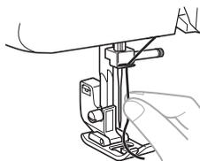
**9** Thread the needle from front to back leaving a thread tail of about 5 cm (2 inches).
