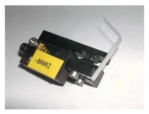
A sensor on a separate arm checks at position +12° that the cigarette has been lit correctly. If this is not the case, the software will eject it before the end of the turn. This sensor has an air connector. Depending on the staining, an additional 4mm OD PU tube can be drawn from the air ducts to the optical sensors to keep this Infrared sensor clean.
