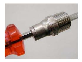
Fig 5 shows how the fitting is tightened (or loosened) from above. Another advantage of the procedure is that prior to inserting the thread the Allen Key will line up the fitting with its thread.
