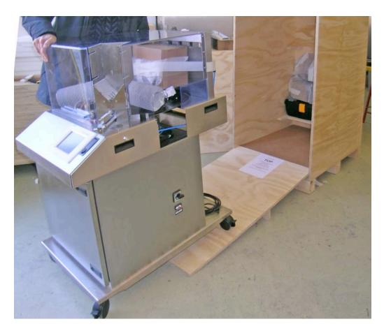
The machine is transported on a 2" expanded polystyrene floor planned to act as a damper in case of shocks during transportation. It is recommended to check that the machine and in particular the stainless steel base plate do not show signs of damage due to vertical shocks (heave).
