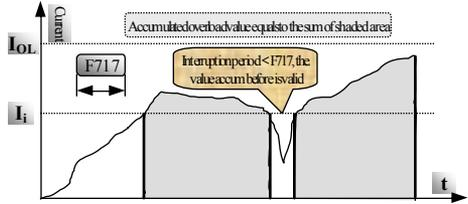
Fig 9-4 Overload Protection
