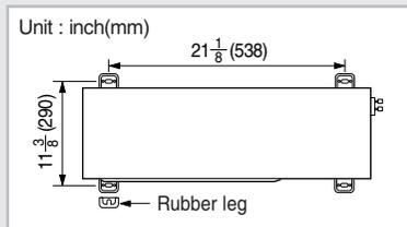
You should install the outdoor unit on a stable base to avoid the generation of noise and vibration, especially when installing the outdoor unit close to your neighbor.
