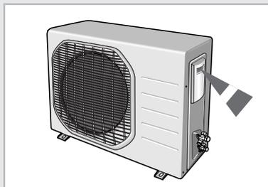
**The outdoor unit is powered from the indoor unit through the assembly cable. If the outdoor unit is more than 24.6ft(7.5m) away from the indoor unit, you must extend the cable. The maximum length of the cable is 49ft(15m).**
