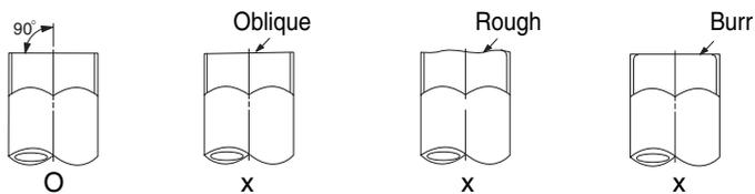
**3** To prevent a gas leak, remove all burrs at the cut edge of the pipe using a reamer.
