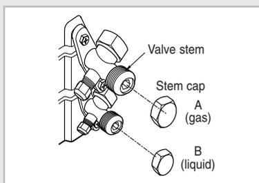
The outdoor unit is loaded with sufficient R410A refrigerant for a 24.6ft(7.5m) pipe. You should purge the air in the indoor unit and in the pipe. If air remains in the refrigerant pipes, it affects the compressor. It may cause reduction of cooling and heating capacity and malfunction. Refrigerant for air purging is not charged in the outdoor unit. Use Vacuum Pump as seen in the picture.
