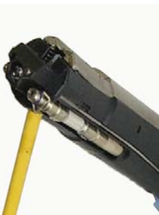
Fig. 3-14 Establishing contact to the heating cartridge
