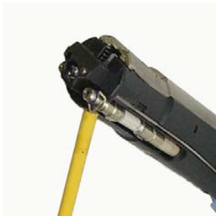
Fig. 3-16 Establishing contact to the heating cartridge
