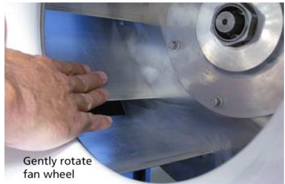
Figure 28: Fan wheel/cone alignment – Step 7a and Step 9a
