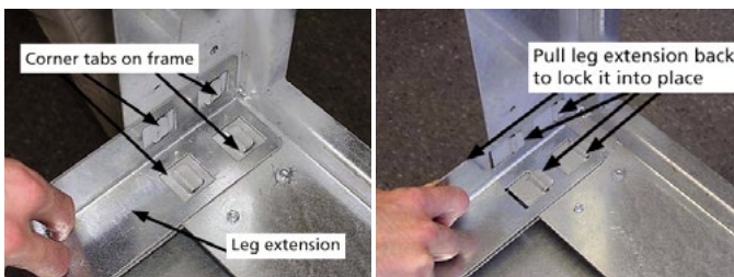
Figure D2: Place leg extensions over the frame tabs, then pull back to lock the leg extension into place
