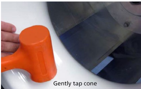
Figure 27: Fan wheel/cone alignment – Step 6
