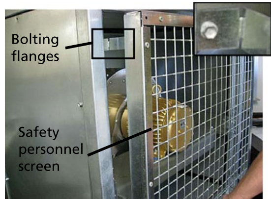
Figure 16: Remove safety screen on motor end
