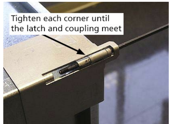
Figure D8: Tighten until latch and coupling meet
