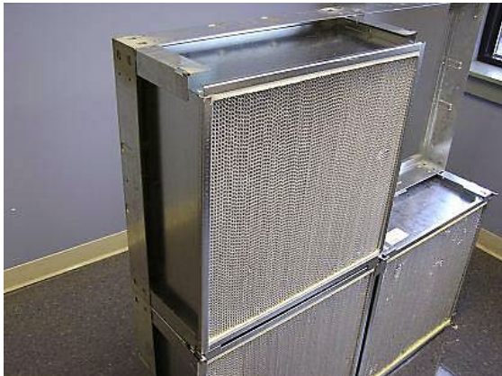
Figure D5: Filter placed inside of frame
