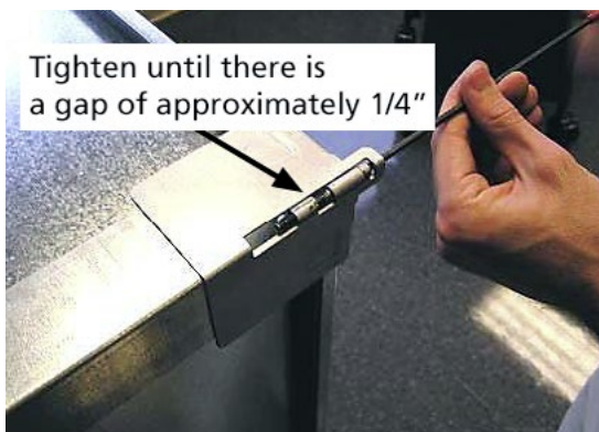
Figure D7: Tighten cap screw to \frac{1}{4} " of the coupling
