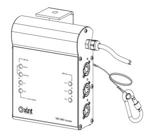
5 way DMX booster, trussmounted. One input, 5 buffered and isolated outputs and one hot output. It has a bracket to mount it onto a hookclamp.
