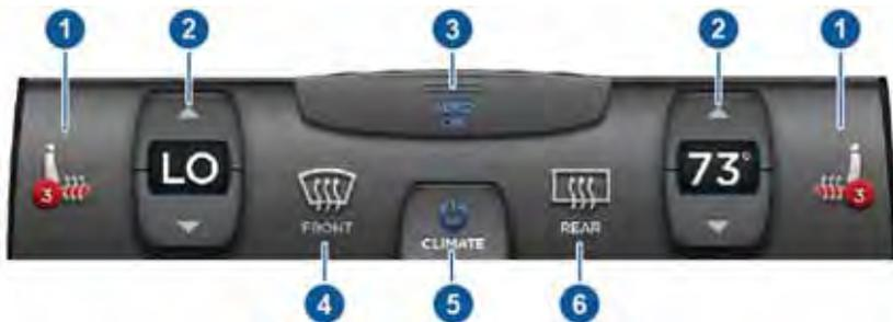
1. The front seats are equipped with heating pads that operate at three levels from 3 (highest) to 1 (lowest).
