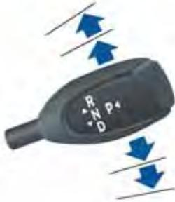
If you try to shift into a gear that the current driving speed prohibits, you hear a chime and the gear does not change.
