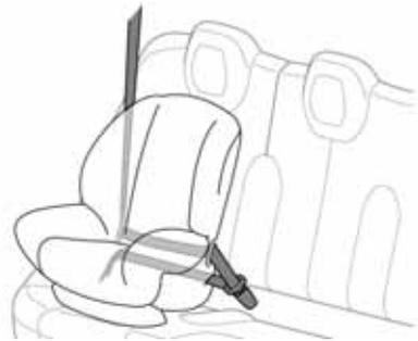
2. Allow the seat belt to retract, and remove all slack in the seat belt while firmly pushing the child safety seat into the Model S seat.
