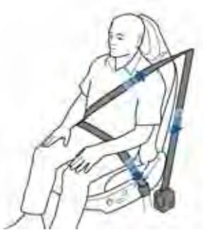
If the pre-tensioners and airbags did not activate in an impact, this does not mean they malfunctioned. It usually means that the strength or type of force needed to activate them was not present.
