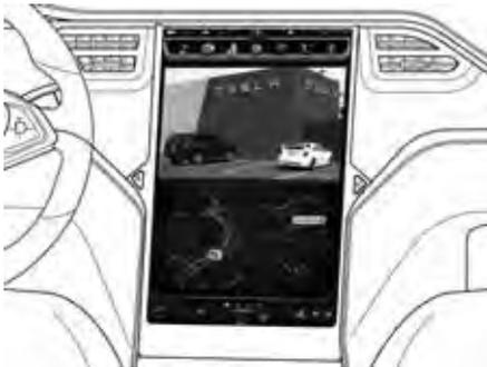
NOTE: If Model S is equipped with the optional Park Assist feature, visual feedback from the parking sensors displays below the camera image. See page 4.16.
