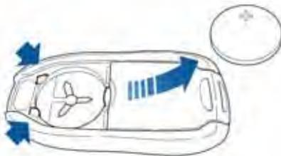
3. Remove the battery by pushing it toward the center of the key to release it from the front retaining clips.
