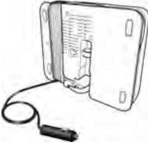
4. Detach the power supply connector from the back of the compressor and plug it into the 12V power socket located on the front of the center console.
