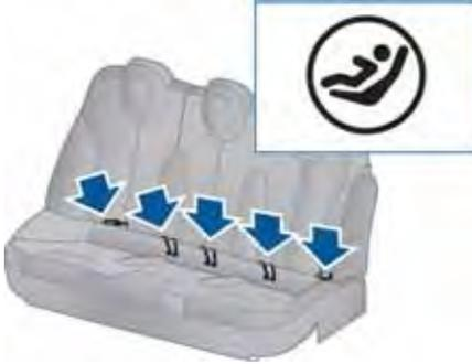
Although ISOFIX anchor points are provided at all three rear seating positions, you can only use two at the same time. To seat three children, use a non-ISOFIX retained seat in the middle. When installing two ISOFIX retained child safety seats, you cannot install them adjacent to each other with one in the middle and the other on the left (driver's side).
