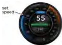
You can accelerate at any time when driving at a set speed in cruise control. But when you release the accelerator, your speed returns to the set speed.
