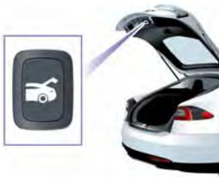
2. Press and hold the button on the underside of the liftgate for 2 seconds until you hear a confirmation beep.
