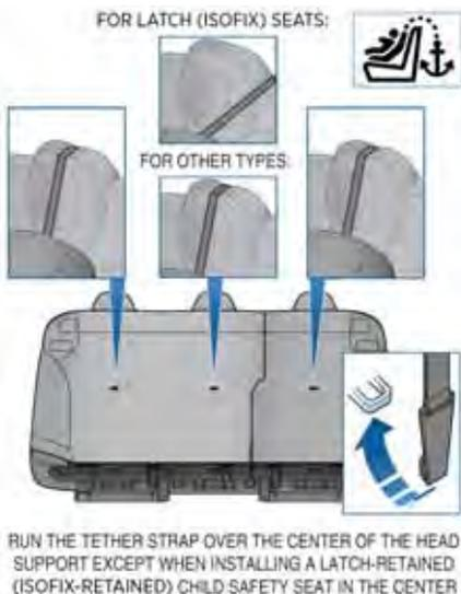
NOTE: To prevent the strap from moving from side to side, the top of the head support deforms.
