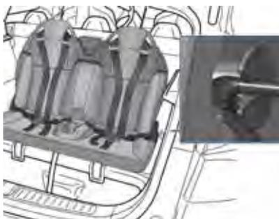
6. Check that the seat back and seat base are securely retained in the upright position by trying to pull the seat back toward you.
