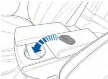
If Model S still does not detect the key, try holding it against the center console, immediately below the 12V power socket (see page 5.16). Or try using another key. If another key does not work, contact Tesla.
