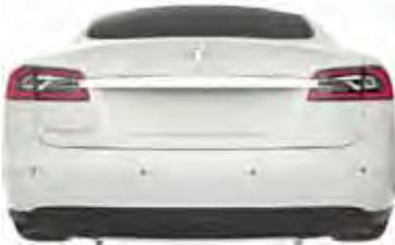
When driving less than 4.8 km/h, the sensors are activated.
