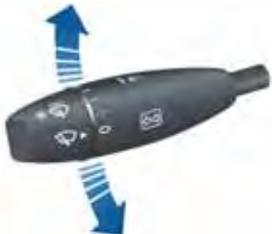
The turn signals stop operating when canceled by the steering wheel, or when you return the lever to the central position.
