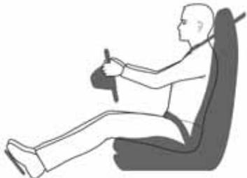
Position the seat so you can wear the seat belt correctly, while being as far away from the front airbag as possible:
