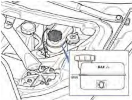
Check the fluid level visually by looking at the outside marks on the side of the reservoir without removing the filler cap.
