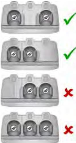
To install a ISOFIX retained child safety seat, slide the safety seat latches onto the anchor bars until they click into place. Carefully read and follow the instructions provided by the child safety seat manufacturer.
