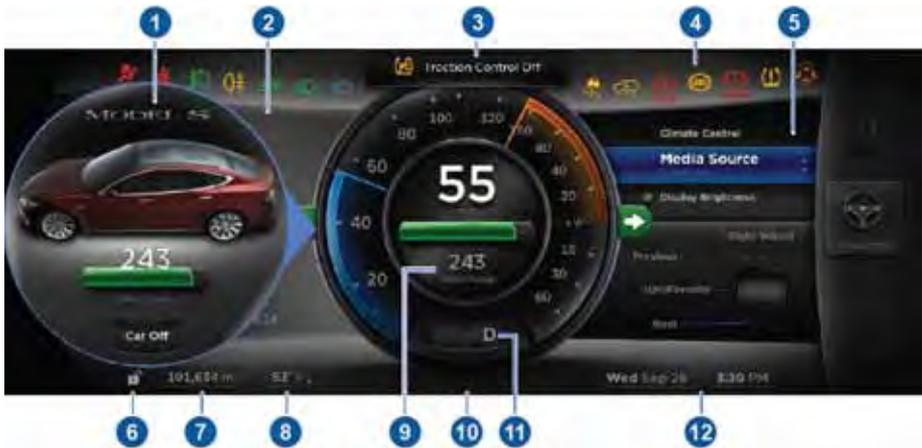
1. The center display changes depending on whether Model S is off or ready to drive. If Model S is off, the center display shows remaining estimated range and status of doors. Pressing the brake powers Model S on—the indicator lights flash on for a second and the center display shows speed, power, charge level, estimated range (see item 9), and active gear. When Model S is plugged in, the instrument panel displays charging status (see page 6.8).
