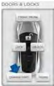
If the cable you are using does not have this button, touch **Controls** > **Charge Port**. Or, you can touch the battery icon at the top of the touchscreen, then from the Charging screen, touch **Open Charge Port**.
