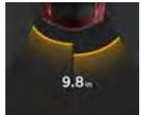
When Model S detects the object within about 40 cm of the front bumper in Drive, and about 30 cm of the rear bumper in Reverse, the red zone and a stop advisory displays. The chime's beep changes to a higher pitch.
