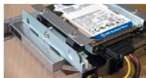
Industrial shock mounts fitted to conventional hard drives
