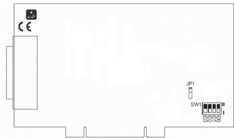
**Figure 3.5: Location of DIP Switch and Jumper on PCI-1758UDO**
