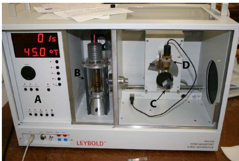
The LEYBOLD X-Ray apparatus: A) is the display and control panel (Note: For this experiment, the controls will be adjusted using computer software.); B) is the X-ray source ( a Molybdenum X-ray tube); C) is the target stage; and D) is the sensor arm.
