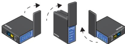
The WiFi antenna is inside the cover. Rotate the cover clockwise to orient the antenna. For best performance, keep the cover vertical when you use your Trek.
