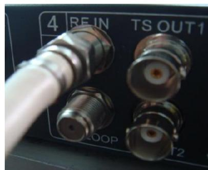
One end is connected to the RF IN interface while the other end is connected to the RF LOOP interface of the next group interfaces:
