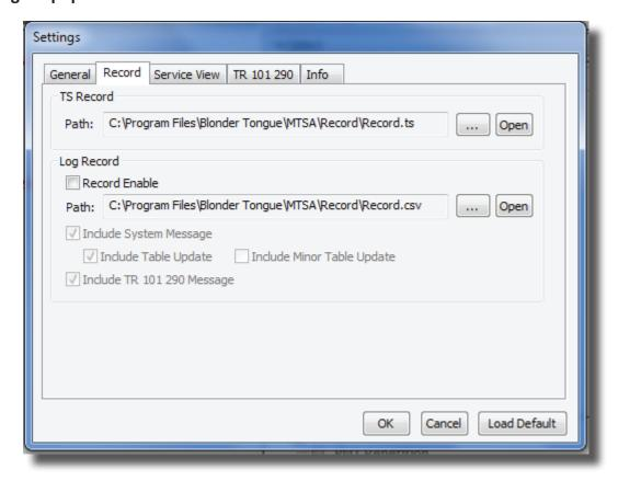
The Record tab facilitates recording streams and logging of system and table messages. Press the Record/Stop button in the Active tab to start/stop recording.
