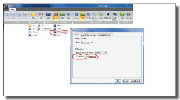
This tab controls the start and stop of the analyzer. Selections are Play, Pause, Stop and Record.
