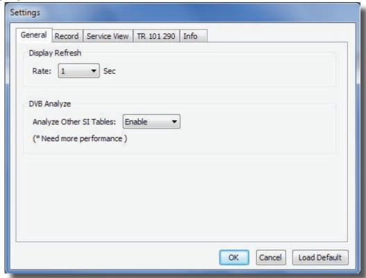
The General tab allows the user to set the GUI update rate. The default is 1 sec. The DVB Analyze option needs a software update before it is fully operational.
