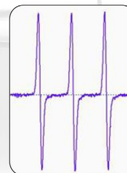
Figure 1: 50 μM aqueous TEMPOL in 1 scan, 1 mm capillary Limit of Detection: 40 nM in PBS
