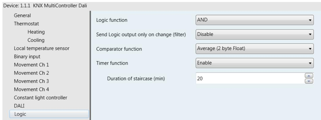
Figure 36 - Parameter window for the logic functions
