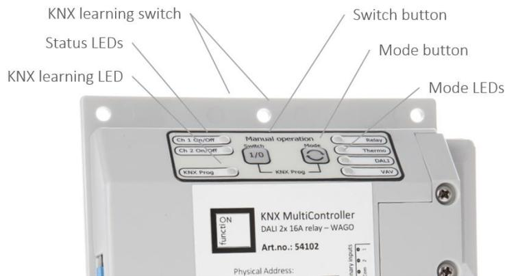
**Figure 3 –KNX MultiController control panel**
