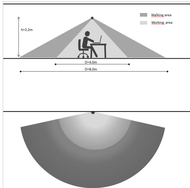
Figure 42 - Detection area for wall mounted sensor (520xx)
