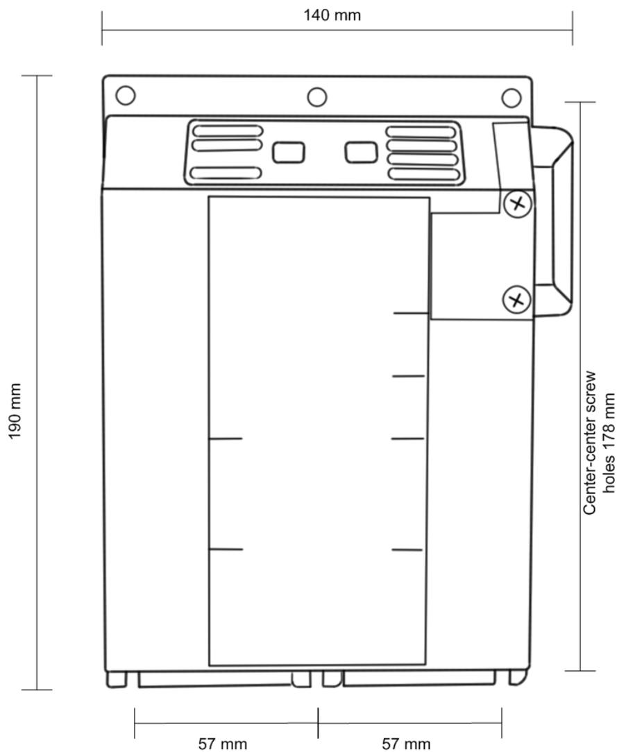
**Figure 37 - Mechanical dimensions of the KNX MultiController (40 x 140 x 190 mm)**
