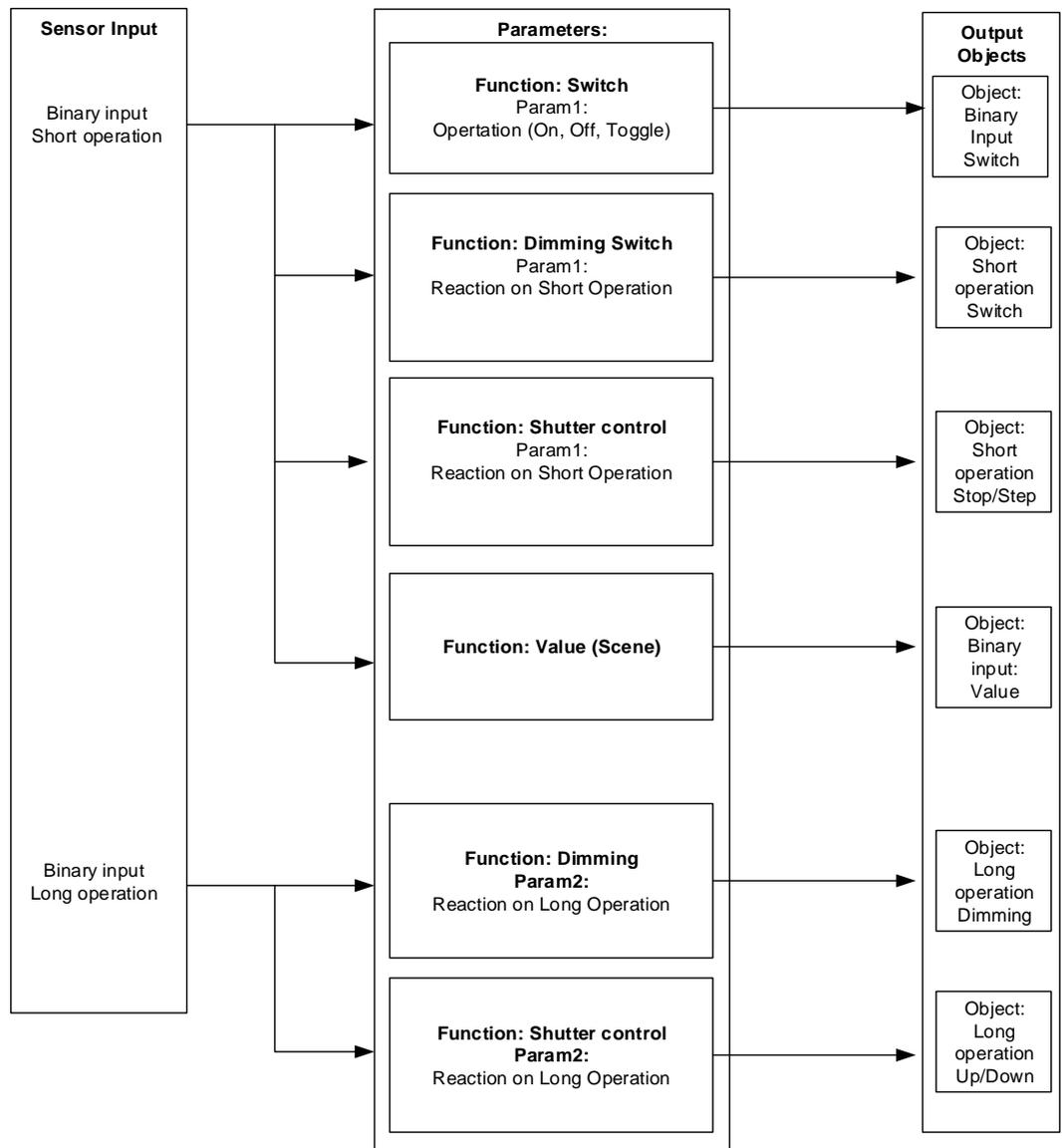
Figure 26 - Block diagram for binary inputs
