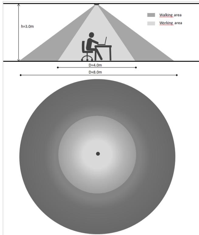
Figure 41 - Detection area for ceiling mounted sensor (520xx)
