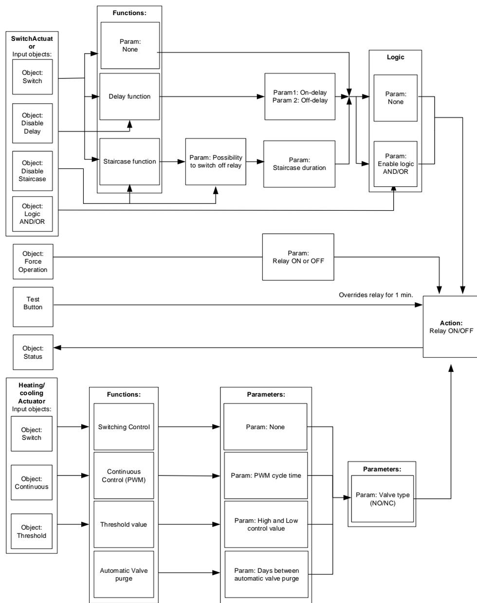
Figure 21 - Block diagram for the switch actuator
