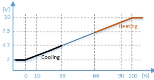
Figure 31 - Output voltage for cooling and heating
