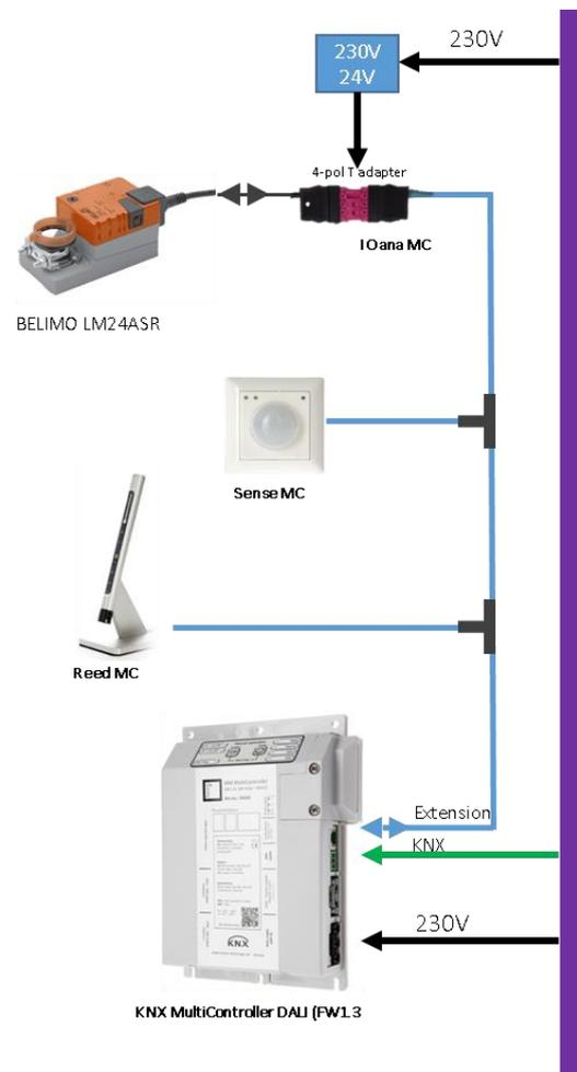
Figure 33 - Typical system configuration (24V VAV motor)
