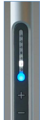
The user panel and IR remote temperature adjustment is by default +/-3°C, but can be limited using set parameters. The adjustment done on the panel will update the "Thermostat: Local adjustment of temp offset" object.
