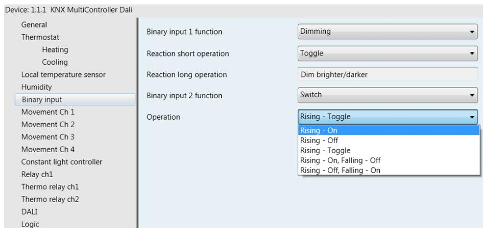
Figure 22 - Configuration options for binary switch input
