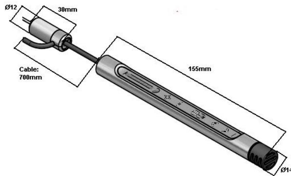
Figure 39 - Mechanical dimensions of Reed panel (155 x Ø14 mm)
