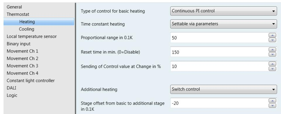
Figure 12 – Additional heating parameter windows, switch control
