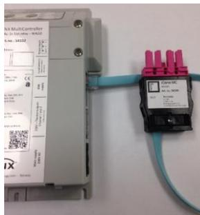
**Figure 28 - MultiController with the IOana 0-10V single input and output extension**
