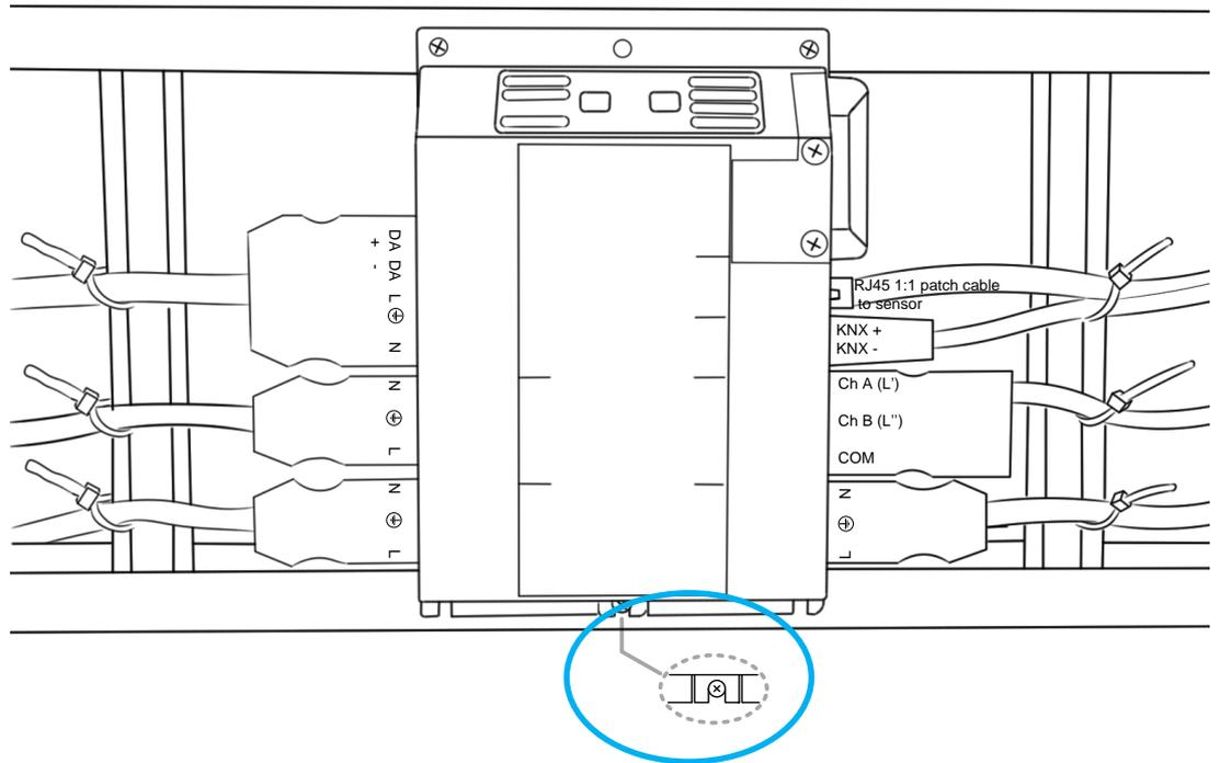
Figure 43 - Typical mounting of the MultiController (seen from bottom side)
