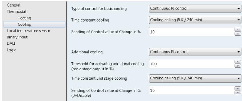
Figure 15 – Additional cooling parameter windows, continuous control
