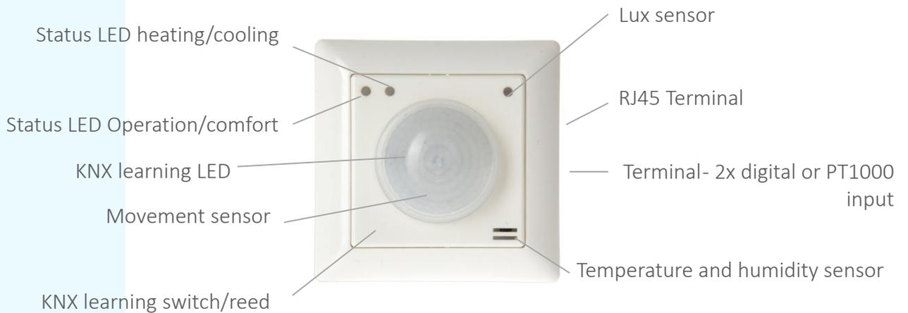
**Figure 2 - KNX MultiController Sensor (52011 or 52021)**
