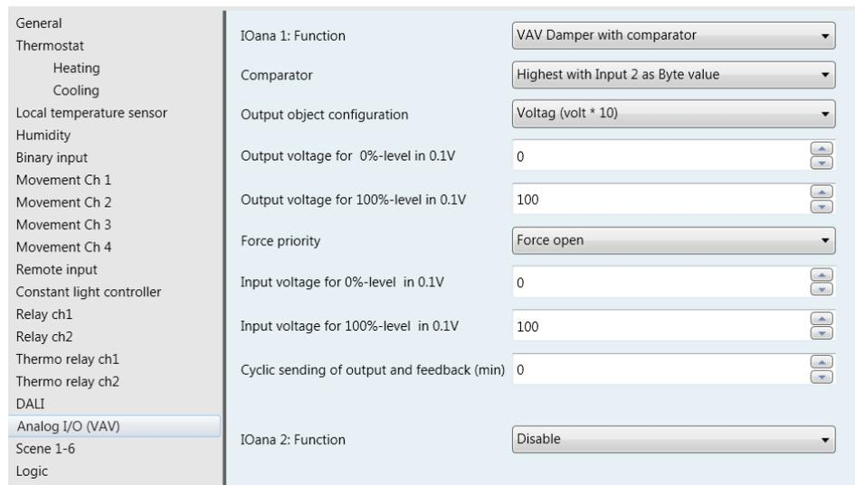
Figure 29 - Parameters for VAV damper control
