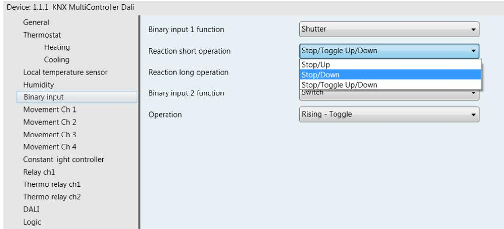
**Figure 24 – Shutter input configuration**
