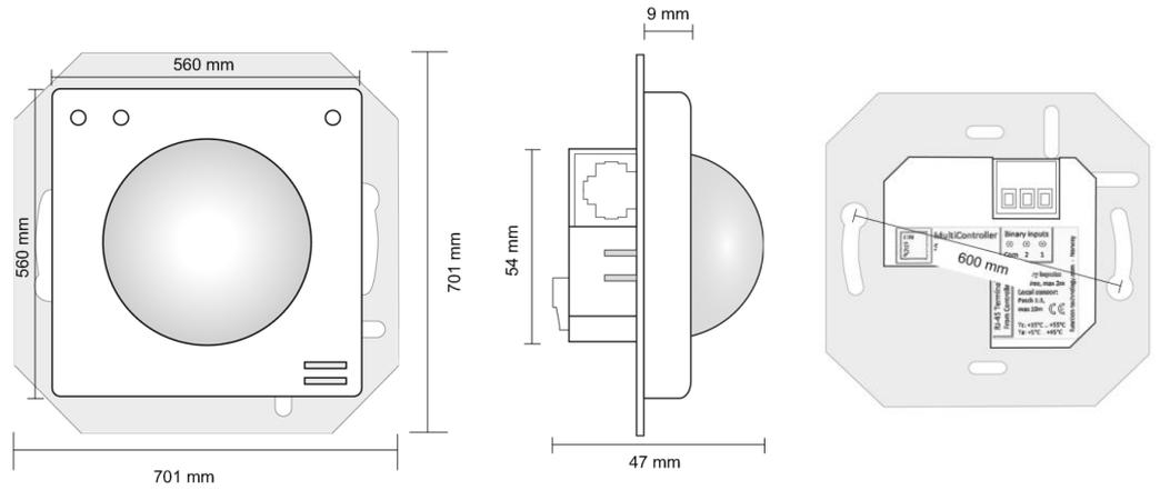
Figure 38 - Mechanical dimensions of the sensor (71 x 71 x 47 mm)
