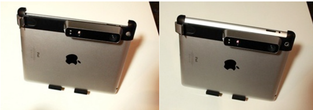
Left: Sliding the bracket on an iPad (4 th Gen). Right: The bracket firmly seated.
