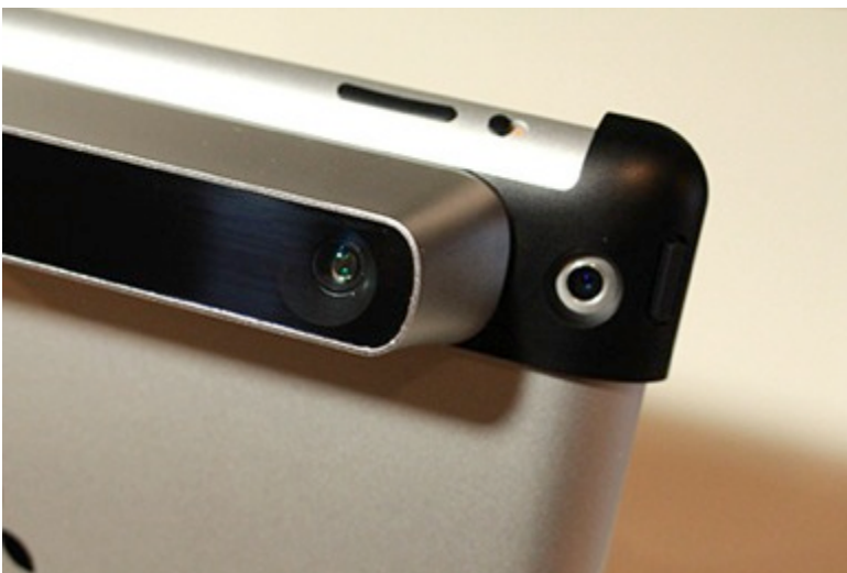
Left: Sliding the bracket on an iPad (4 th Gen). Right: The bracket firmly seated.
