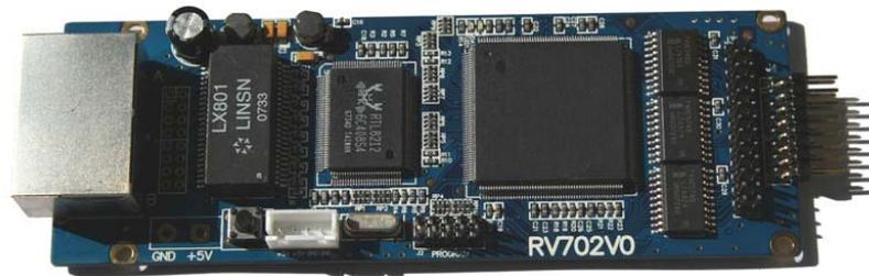
Receiving card is building-in inside of each cabinet. The function is to receive data from sending card via Cat5 cable, then transfer data to led display signal. 5V power supply is required as well. The necessary setup is needed when a new receiving card is placed.
