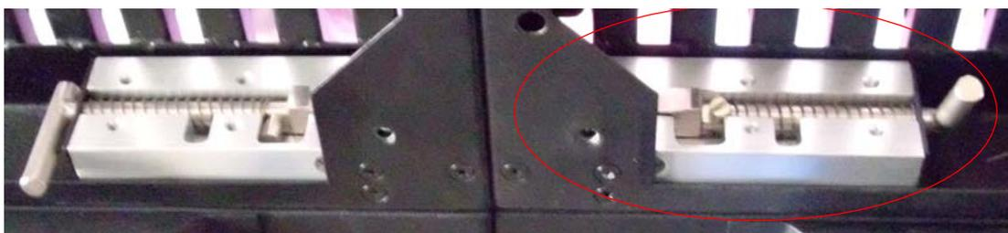
As shown before, P18 LED curtain contains two fast locks on each side of the bottom. The ROPIX P18 needs to use these two fast locks to fix all panels on vertical.
