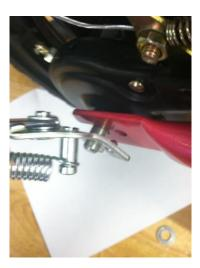
NOTE: If the dimple does not line up with the hole then loosen the screw that attaches the brake component to the frame. Slide the wheel to where the kickstand fits properly and tighten axle nuts, and then retighten the screw. Also, if your kickstand appears to be too long, simply pull the bottom of the kickstand away from the bike while attached, bending the stand about a half of an inch away from the bike.
