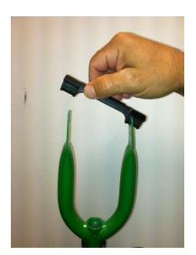
Insert the wheel into the fork and replace the hook washers onto the axle so the tab fits into the corresponding hole, then put on flat washer and tighten the axle nuts with the provided tool.
