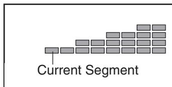
of the matrix. (The incline settings are not shown in the matrix.) The speed settings for the next seven segments will be shown in the columns to the right.
