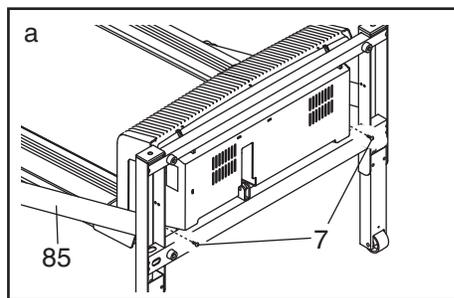
b. Raise the Uprights (85) to the vertical position. Remove the three Screws (7) from the Hood (33), and carefully pivot the Hood off.
