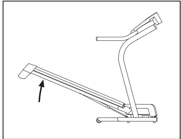
2. Move your right hand to the position shown and hold the treadmill firmly. Using your left hand, pull the latch knob to the left and hold it. Raise the treadmill until the frame is past the pin on the latch knob. Then, carefully release the latch knob. **Make sure that the frame is held securely by the pin.**
