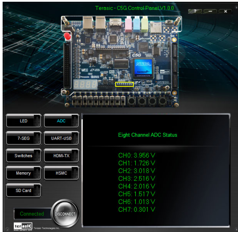
Figure 2-8 Reading of eight channel ADC
