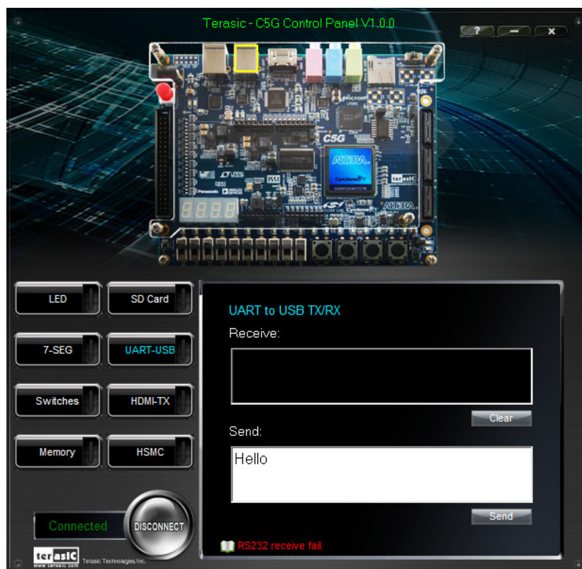
Figure 2-9 UART to USB Serial Communication
