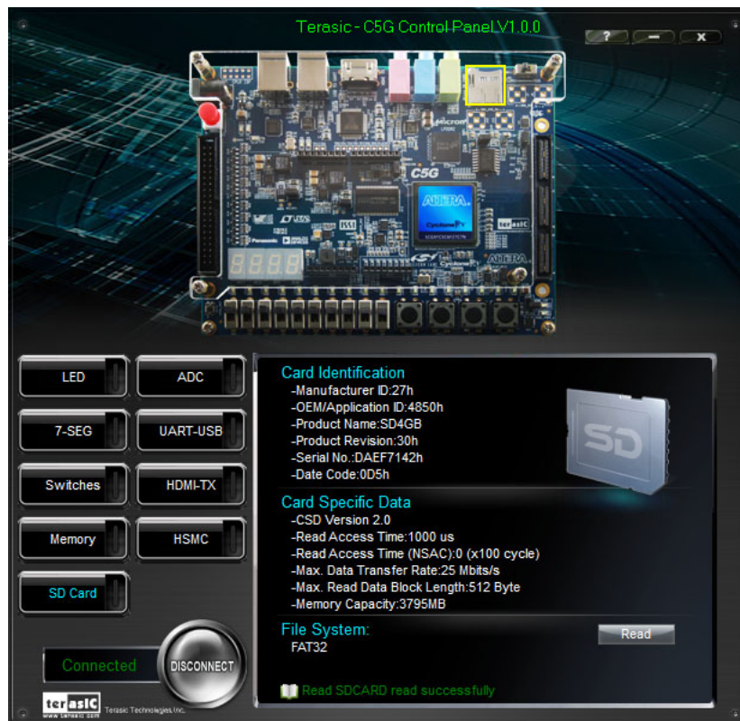
Figure 2-7 Reading the SD Card Identification and Specification
