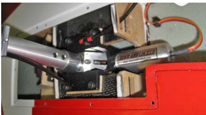
Converted gear mounted in the wing.
