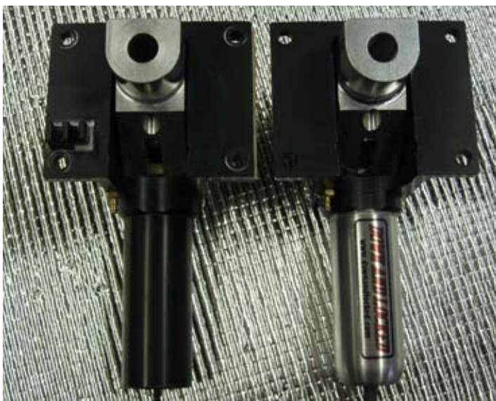
Before and after: The stock gear is on the left, Down and Locked converted gear is on the right.
