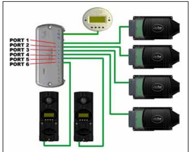
When first powering-up the system, make sure all of the OutBack products are plugged into the HUB and powered before plugging the MATE into the HUB.
