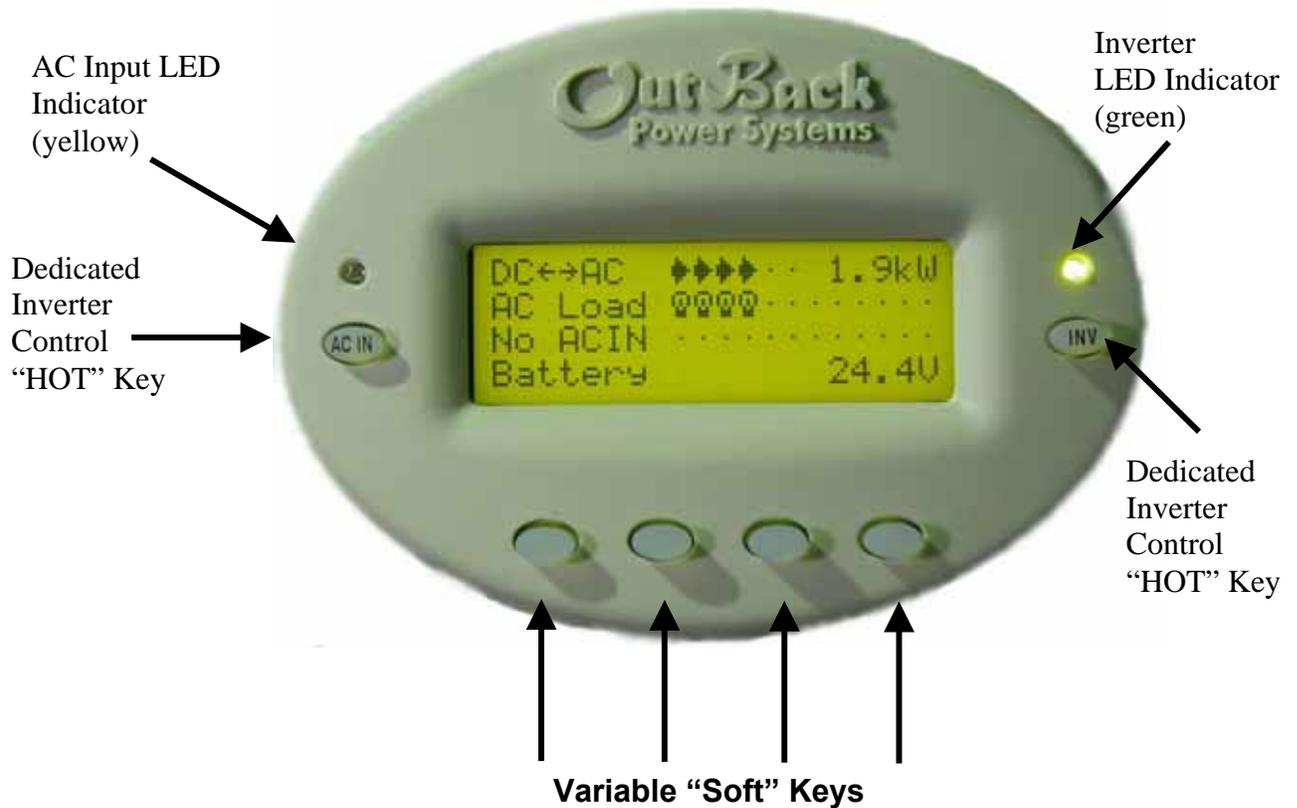
*each one of the soft keys corresponds to a word on the bottom line of the LCD display*
